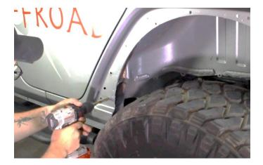
With an M8 Nutsert Tool, install a nutsert into each of the drilled holes.
