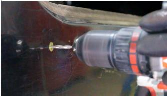
Using some silicon or paint, touch up the sheet metal you just drilled through to prevent rust. We recommend using a Q-tip for application.
