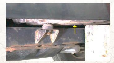
In the approximate location shown above, use a jack to lift your body away from the frame. You only need to lift a small distance to allow enough room to slide the new rock slider in place.
