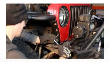
Loosely attach the rear of the fender to the OEM bolt locations on the body tub and the lower inner fender.
