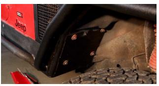
Once clearances have been checked and you're good with the fit, tighten the hardware on the front and rear of the fender.
