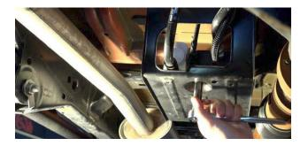
To the right of the electrical connector on the rearmost end of the EVAP canister, remove the upper hardline using two small flat head screw drivers. You will use one screw driver on each side of the c-clip. Each tab must be pried open while simultaneously pulling the clip away.
