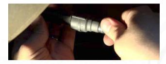
The two hardlines on the passenger side will require that you have the c-clip loose when you insert the hardline into the canister connectors. Once you've pushed the hardlines in place, press the c-clips into position to lock the lines.
