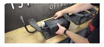
Slip the hardline through the rear of the Fishbone Offroad EVAP canister skid plate. Ensure the mounting tab for the canister is towards the bottom of the skid plate so it can be bolted down.
