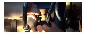
On the left side of the EVAP canister is another hardline that connects to the white plastic housing. Follow this hardline up to the connector about 12" away. Disconnect this hardline by moving the release tab clockwise with your thumb, while pulling the connector apart. Again, view our installation video for a better visual of this step.
