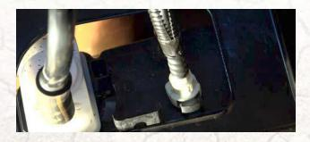
Remove the electrical connector by pressing the locking tab in on the connector and carefully disconnect it.
