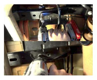
Remove OE skid plate and canister from the vehicle.
