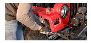
Mark a straight line up the inner back portion of your fender. This should be 1" from the outside edge of the factory fender. Again, ensuring there are no obstructions, cut along this line.
