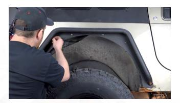
Align your new fenders with your Jeep's body and tighten with the supplied washers and nyloc nuts.
