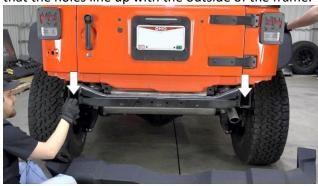
With the help from a second pair of hands, lift the bumper up to the frame of the Jeep. Using a short 12mm bolt, lock washer, and washer, loosely fasten the bumper brackets to your frame rail. Do not tighten yet, as you may need to adjust the bumper when installing the other bolts.
