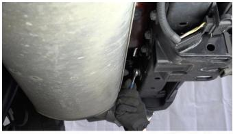
Remove the 2 16mm bolts between the body and bumper.
