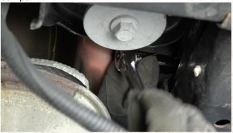
If your vehicle comes with a recovery hook, it will need to be uninstalled by removing the 3 18mm bolts.
