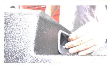
If your model has sensors, pop out our included sensor plugs from the bumper, and re-install your sensors in order, and as they were oriented in the factory bumper.
