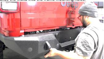
With the included flat washers, lock washers and hex nuts, secure the bumper to the left and right frame mounts with an 18mm Socket.
