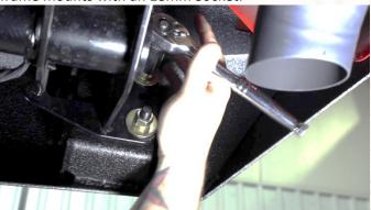
With the included tapered bolts, washers, lock washers, and nuts, secure the center of the bumper to the center frame mount.
