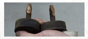
Reinstall all body mount bolts and torque to factory recommended specifications.
