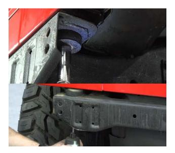
Again, using the 5/8" socket, remove the bolts that secure the body mounts in front of the gas tank.
