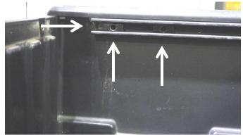
Your vehicle may or may not have a front trail rail, but will come with be bolts in either case. These bolts will be used for this installation. If you do have the rail, with a T-30 torx bit, remove the 5 bolts and washers, and remove the rail.
