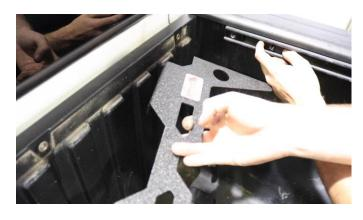
Line up the bracket with the front wall holes, and secure it with 2 of the factory bolts and washers, with a T-30 torx.
