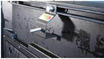
Lift the jack over the bolts, and secure it with the 2 included wing nuts.
