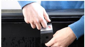
Determine the spacing needed for your jack. Once you're satisfied with the bracket location, secure the bolts with a 19mm socket.
