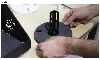
Next, remove your vehicle's spare tire and place the tire mount onto the carrier's studs, so that they rest evenly in one of the 3 smallest fitting holes.
