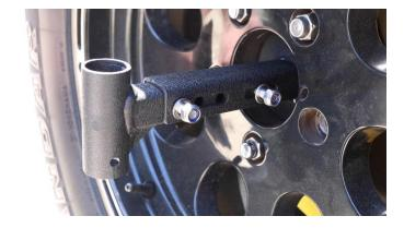
Finally, insert your desired flag pole into the mount and secure it with the included Lock Pin.
