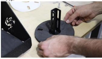
Next, remove your vehicle's spare tire and place the tire mount onto the carrier's studs, so that they rest evenly in one of the 3 smallest fitting holes.
