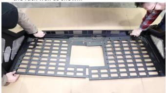
Follow the perimeter and loosely secure every bolt point with M6 bolts, washers, and Nyloc nuts. Including the middle joined plates.
