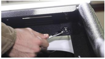
Begin securing the rack to the bed. Put 2 of the M12 carriage bolts through the bracket as shown, and rotate it into the side panel bracket, and up into the bed rail. With 2 flat washers, lock washers, and hex nuts, tighten the two brackets down onto the plastic rail with a 19mm socket.
