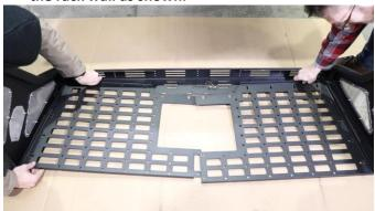
Follow the perimeter and loosely secure every bolt point with M6 bolts, washers, and Nyloc nuts. Including the middle joined plates.
