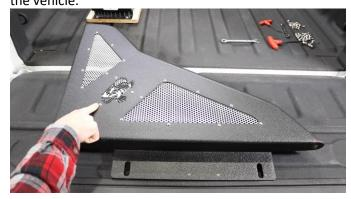
Begin applying the adhesive foam to the panel and panel brackets for both side panels.
