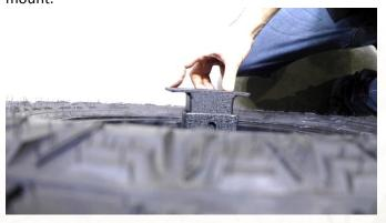
Completely tighten down the 3 hex bolts.
