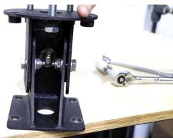
Hold the mount up to your tire and adjust its length so that the mounting plate is flush or near flush with the tire, ensuring that it will lie properly on the mount.
