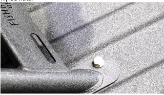
With the help of a friend, tighten down and secure the carrier with 2 19mm sockets.
