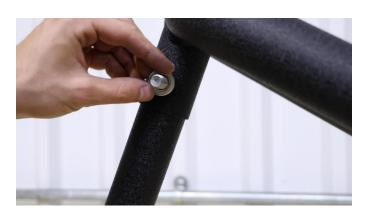
With the hub mount and frame, secure the two with 4 M12 bolts, 4 M12 washers, 4 oversized washers, 4 Nyloc nuts, and 2 19mm sockets.
