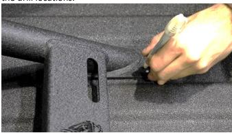
\*Again, ensure that drilling below these points won't damage vital components\*
