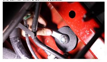
Place your tire onto the carrier and secure it with its lug nuts, or the 3 we've provided.
