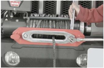
With a 5/16" Allen wrench or hex bit socket and an 11/16" wrench, secure the Fishhook with a lock washer, followed by a nut.
