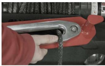
Holding the two parts together, place them up to your bumper and into place using the two included bolts lead by a flat washer.
