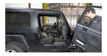
Lift your door straight up to remove the pins from the hinges. You may need to rock the door back and forth to get it to lift out. Store your doors in a safe place against a blanket or cardboard to protect the paint.
