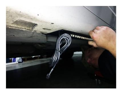
3. After you decide the locations to place the screws remove your Rocker Panel and begin drilling the necessary holes.
