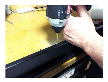
4. Now you need to simply mount the Rocker Panel onto your vehicle in the desired location with the mounting screws.
