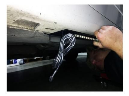
3. After you decide the locations to place the screws remove your Rocker Panel and begin drilling the necessary holes.
