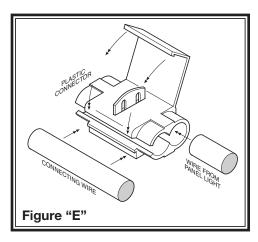
connector over the existing wire and insert the un-stripped wire from the pressure switch into the wire connector. Close the wire connector over both wires with pliers **see Figure "E"**.
