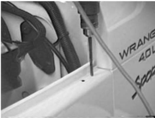
Drilling Mount Holes
