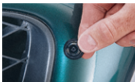
Adhere Stick-a-Stud™ fasteners to vehicle
