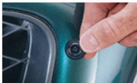
Adhere Stick-a-Stud™ fasteners to vehicle
