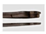
APPEARANCE: One or more brake pad within the axle set will be excessively worn
