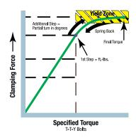
Fel-Pro® engineers suggest technicians use a gauge such as the affordable Fel-Pro Torque-to-Angle Indicator (part number TRQ-1). It fits easily on the 1/2" drive of a torque wrench and eliminates uncertainty about the additional torquing required for T-T-Y head bolts.
