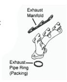
gaskets for flange-to-flange connections.
