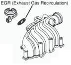
are burned in the combustion process. A leaking EGR valve gasket can allow exhaust gases into the engine compartment and unwanted air into the intake manifold. Replacement of this gasket is necessary during EGR system service.
