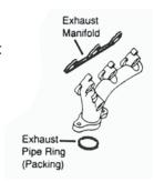
gaskets for flange-to-flange connections.
