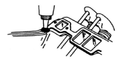
**PRIOR TO REINSTALLING INTAKE MANIFOLD** apply a small dab of silicone sealer to the 4 corner intersections between the end seals and gaskets.
