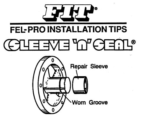
To insure proper function of this product on this application this sleeve must be aligned perfectly, straight and true and fully bottomed on the balancer hub before assembly.
