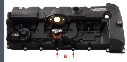
EN Attention: Loosen the two bolts of holder A before tightening the valve cover. Note: Only when the two bolts (B) have been tightened to the manufacturer's specified torque of 9Nm can the two bolts of holder A be tightened again with a torque of 5Nm.
