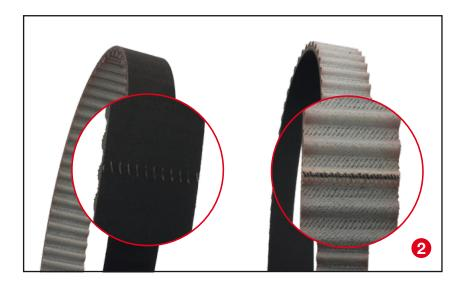
The demands on timing drives are constantly increasing. The result is the continuous refinement of timing belts. Some timing belts are Teflon coating. The coating helps to reduce friction and wear which extends the belt's service life particularly in high-performance engines. The coating may vary in colour (see Fig. 1) although the colour has no significance and no effect on functional capability.
