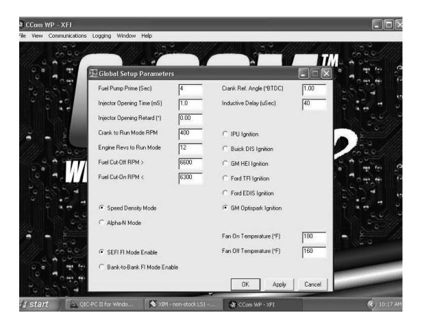
Note: As with any distributor installation, use a high-quality timing light to verify ignition timing matches the timing advance commanded by the  $XFI^{TM}$ . If necessary, make slight adjustments with the distributor to correct this.
