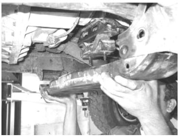
4. Remove the two bolts that hold the factory trans bracket to the trans mount. Remove the four bolts that secure the trans mount to the transmission. Raise the jack just enough so that the stock mount can be removed. SEE PHOTO ON NEXT PAGE
