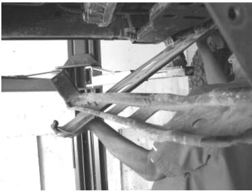
3. Remove the two transmission mount nuts from the crossmember. Carefully raise the transmission and remove the four crossmember bolts from the frame saving the crossmember and the hardware. SEE PHOTOS IN NEXT COLUMN
