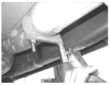
6. Locate FT44116 Drop Transmission Bracket and factory hardware. Install the new mount onto the trans and then the mount onto the trans bracket. Re-install the crossmember. Lower the transmission and reinstall the factory flange nuts securing the trans mount to the crossmember Tighten all of the nuts and bolts. Lower the jack that was used to support the transmission and torque all of the hardware to 95 ft. lbs. Re-tighten the exhaust clamps. SEE PHOTOS BELOW.
