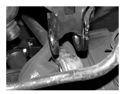
4. Locate the lower pivot ball joint assemble at the axle end of the track bar. Remove the nut attaching the bar to the ball joint in the axle. Retain the factory hardware and discard the factory Track Bar **SEE PHOTO BELOW.**
