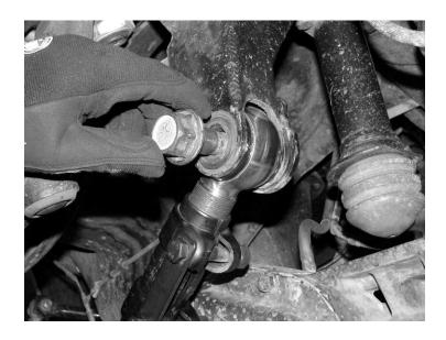
7. Center the axle accordingly using the adjuster sleeve on the track bar. After all adjustments have been made lock down the adjuster sleeve with the cross bolts. It is important that the sleeve is locked down with cross bolts perpendicular to the diff cover. **SEE PHOTO BELOW**
