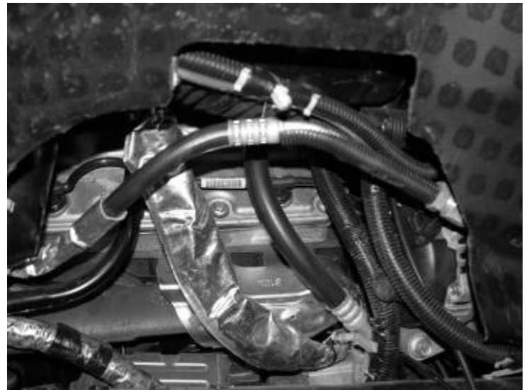
Photo shows bent A/C line
