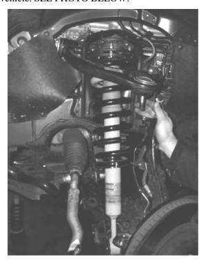
5. Remove the front and rear lower control arm compression bump stop pads with a strap wrench and install the supplied FT89034 spacer between the pad and the frame. SEE PHOTO BELOW.
