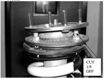
8. Install coilover on the truck starting at the top. Torque nuts to 30 ft.lbs. SEE PHOTO BELOW.
