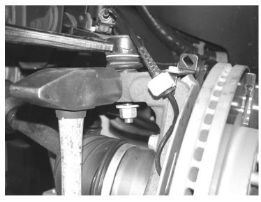
4. Loosen the tie rod nut and strike knuckle with hammer till it comes loose. Save all hardware (Use care not to hit threads.) Disconnect the factory swaybar endlinks and save with the hardware. SEE PHOTO BELOW.
