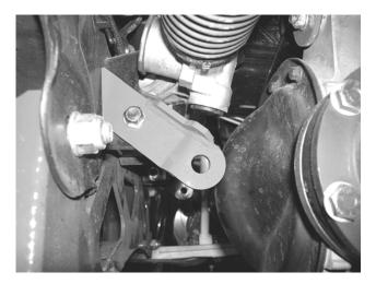
3. Working from the passenger side of the truck, locate the factory rack and pinion frame mount and remove the bolt horizontal to the frame. Following the drawing below cut the corner of the frame bracket back 1" using a die grinder. Locate FT30084 Passenger side frame bracket and attach it to the frame using the supplied 12mm x130mm bolt, nut, and washer. Note: On the FT30084 bracket the side with the washer welded to it will be against the frame. Torque bolt to 70 ft. lbs. SEE DRAWING BELOW.
