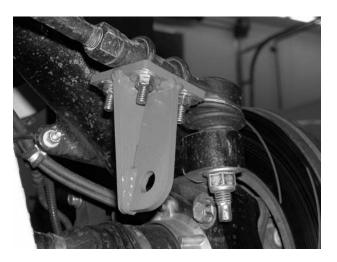
5. Locate FTS7004 or FTS6602 Steering Stabilizer. Attach the stabilizer to the frame bracket and to the tie rod end bracket using the supplied bushing and hardware. Torque nuts to 25 ft. lbs. SEE PHOTO BELOW.
