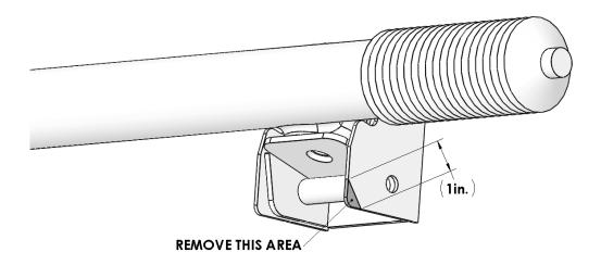
4. Working from the driver side of the truck, locate FT30078 tie rod end bracket. Using the supplied FTS31UBK u-bolt kit attach the tie rod end bracket to the tie rod end. When attaching the tie rod end bracket to the tie rod end you will want to place the bracket at the end of the tie rod, against the jam nut. Torque u-bolt nuts to 25 ft. lbs. SEE PHOTO BELOW.
