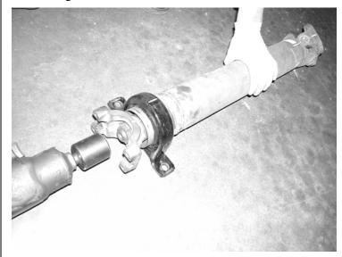
**9.** Re-align the marks on the front of the drive shaft with the transfer case flange and re-install the factory hardware. SEE PHOTO BELOW.
