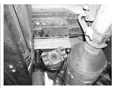
**11.** Re-align marks on front and rear drive shaft halves and re-attach with factory hardware. SEE PHOTOS BELOW.
