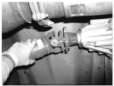
**10.** Install required FT419 Carrier Bearing Shim Kit at this time and re-attach carrier bearing to the frame cross member. SEE PHOTOS BELOW AND NEXT COLUMN.
