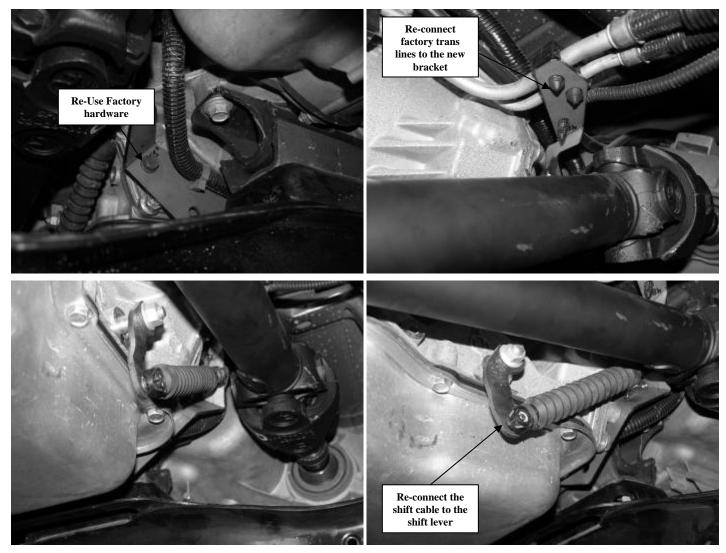
3. Install the driveshaft into the t-case first and then attach the front differential with the factory hardware. Torque the bolts to 18 ft. lbs.
