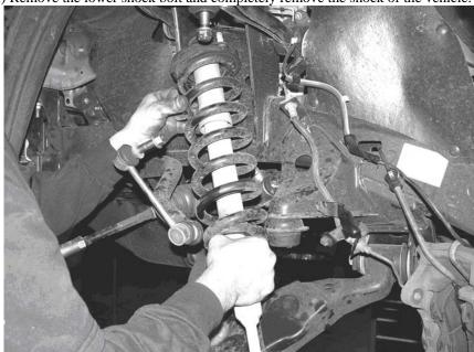
7.) Now move to the passenger side and repeat the procedures in removing the stock shock of the vehicle.
