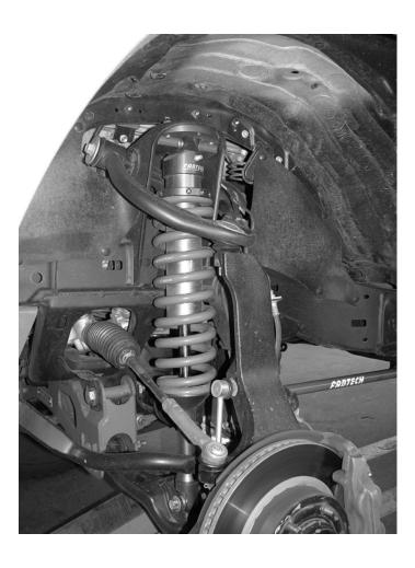
4.) Now move to the passenger side and repeat the procedures for the installation of the Coilover. Once both sides have the newly installed Coilover, reinstalled the sway bar links on both sides and also reinstalled the tie rod ends. You have now completed your installation. Spanner wrench is not included in this kit if needed order FTS98008. We recommend driving the vehicle for 50 miles and retorque nuts and bolts and then have it aligned to factory specs.
