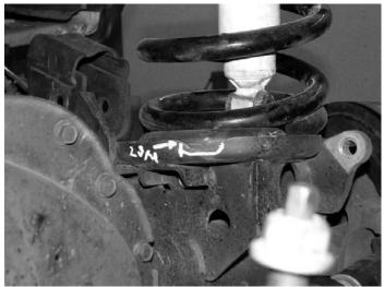
15. Connect the track bar to the new drop bracket using the supplied 9/16" x 3" bolt, nut, and washers. **NOTE: This may need to be done when the truck is back on the ground.** SEE PHOTO BELOW.
