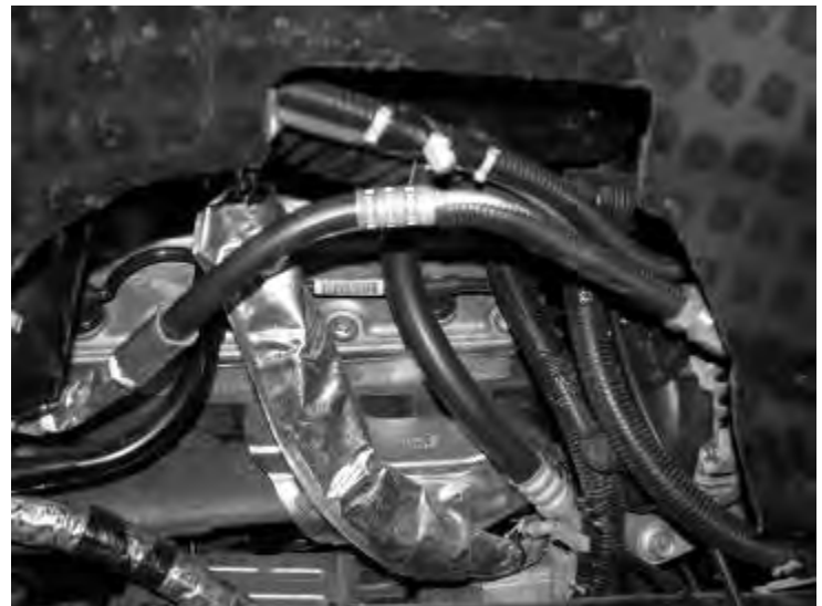
Photo shows bent A/C line
