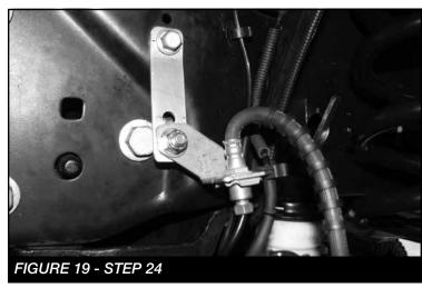
25. (PASSENGER SIDE) Install FT30659 (Brake line bracket) to the factory brake line tab using the supplied 3/8" hardware (Use lower hole). Next, using the supplied rubber clamp and 1/4" hardware, attach the ABS line to the upper hole on the FT30659 bracket. Re attach to the frame using the factory hardware. Torque 3/8" & factory hardware to 52 ft-lbs. Torque 1/4" hardware to 14 ft-lbs. SEE FIGURE 20
