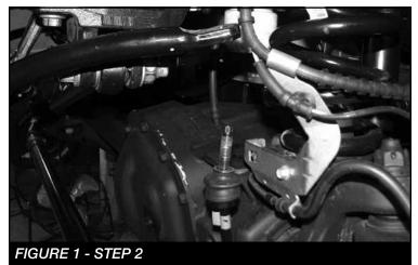
Disconnect the brake line from the frame and axle on both driver and passenger sides. Save hardware. SEE FIGURES 2-3
