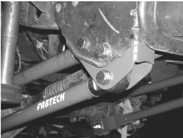
Assembly of the FT292 Alignment Cam
