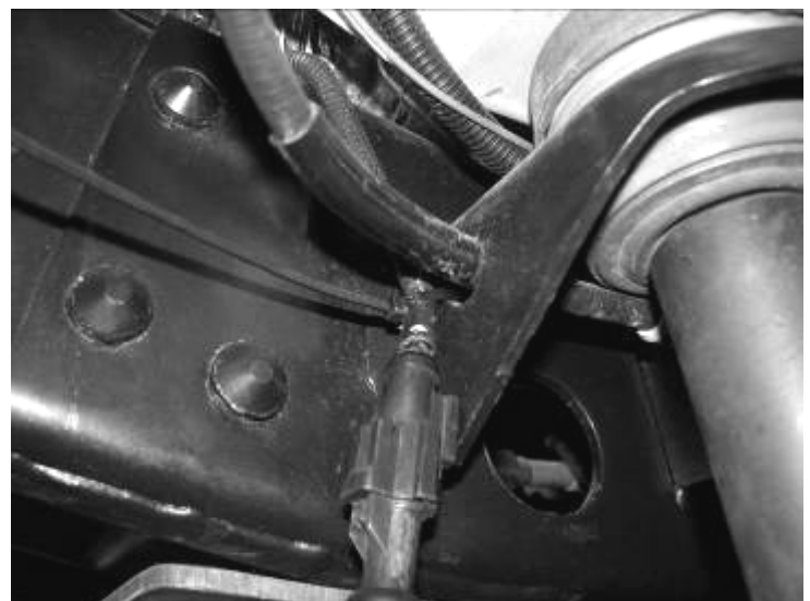
Picture Shown with Factory Stabilizer re-installed
